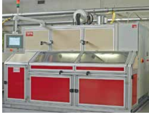
Burst test stand capable of performing burst tests on hose assemblies up to 10.000 (145000 psi)
